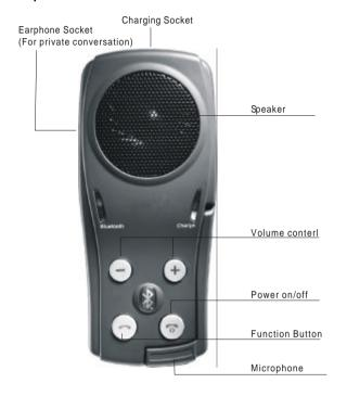
**Function Button:** Performs several interrelated functions. **Microphone:** Built-in type on swivel arm (30° is the recommended angle. See picture on front cover)
